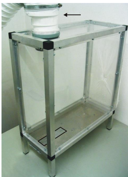
Fig. 2: ATC (side view). The air ventilation system is connected to the cage (black arrow). The arm is exposed at the test window in the metal floor sheet (black rectangle). The rear side is covered by gauze.
